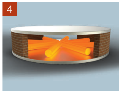
4 Heating of billet in rotary furnace
